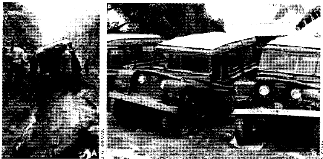
Plate 18.2. A: The protracted fighting in Zaire devastated the road system, and vehicles frequently became mired along bush trails. B: Broken chassis were common; without a special repair and maintenance workshop, the programme would have foundered.
